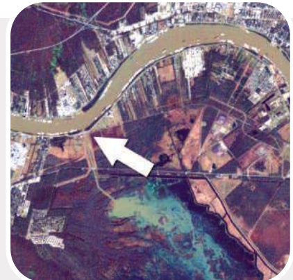
Test run. In early trials, sediment (brown) passes from the Davis Pond structure (arrow and detail below) into Lake Cataouatche.
